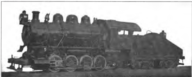
Fig. 20. Eight-Wheel (0-8-0) Switching Locomotive. Built by the American Locomotive Co. for the Chesapeake & Ohio. Cylinders 21 in. x 28 in., Working Steam Pressure 200 lbs. per sq. in., Heating Surface 2,705.1 sq. ft., Diameter of Drivers 51 in., Weight on Drivers 171,175 lbs., Total Weight 171,175 lbs.
